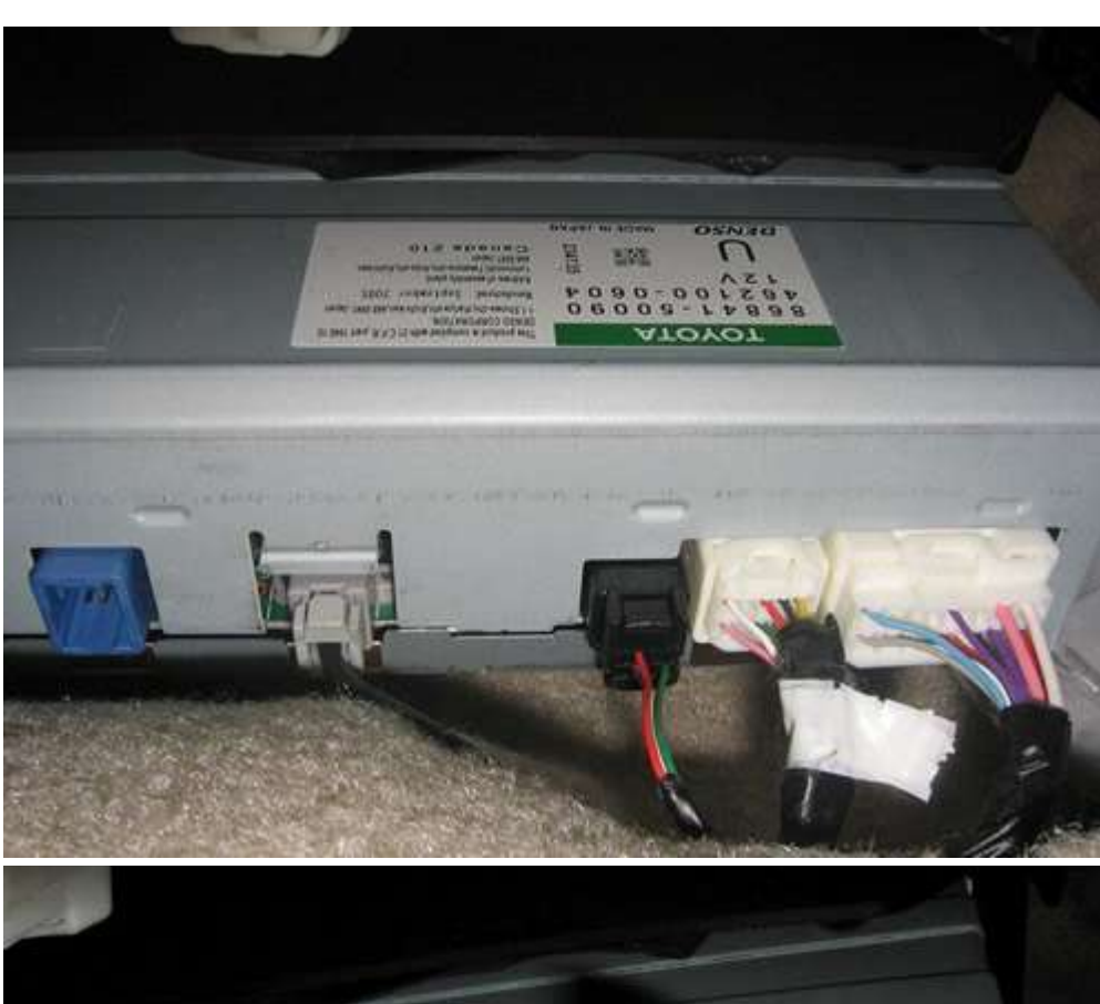
1) This is the Toyota Prius 2005 Navigation system box located under the driver's seat, prior to the install. This is the view looking from the driver's foot well (from the front) Note the grey wire on the bottom left of the right connector (N2)
