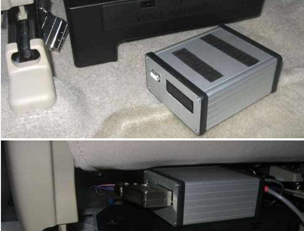
5) View with velcro on base of CAN-view and matching velcro on NAV box.
