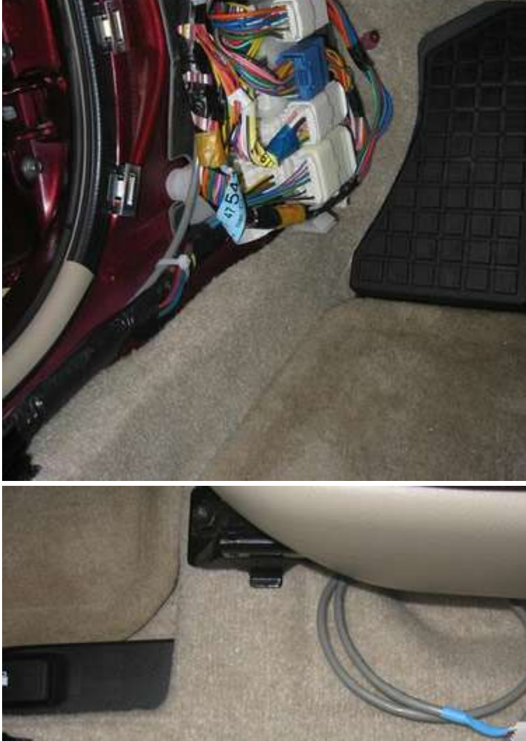
18) Cable goes down thru the kick panel area into door sill.
