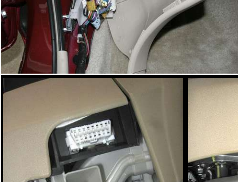
12) Driver's side kick panel removed exposes wiring
