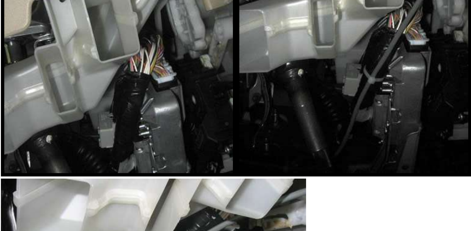
13) (left) OBD2 connector under dash to right of steering wheel 14) (right) Connected cable to the OBD2 connector and routed back
