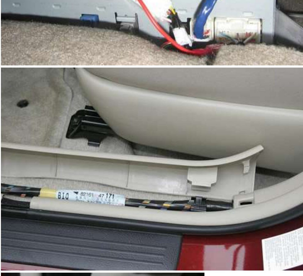
9) Installed CAN-View on top of NAV (view from front) This view is from the front with the driver's seat all the way back. Note that the seat wiring and connectors come back and gently touch the CAN-View box as long as the CAN-View box is mounted all the way to the rear of the NAV box. If the CAN-View were further forward it would impact the seat connectors when the seat goes back
