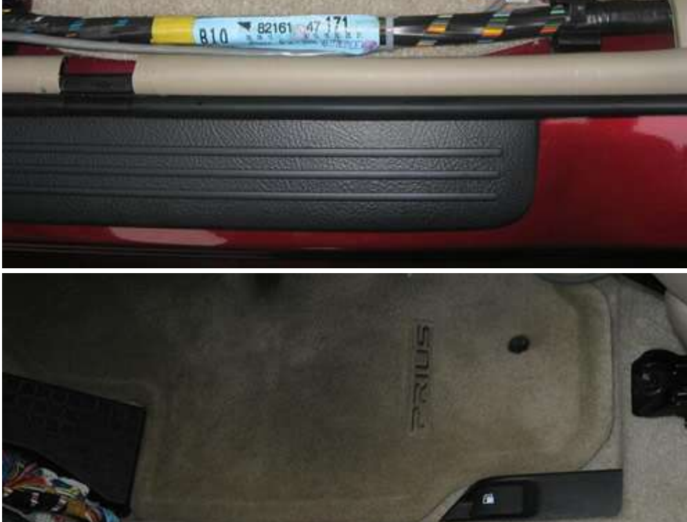
19) Cable runs along door sill.
