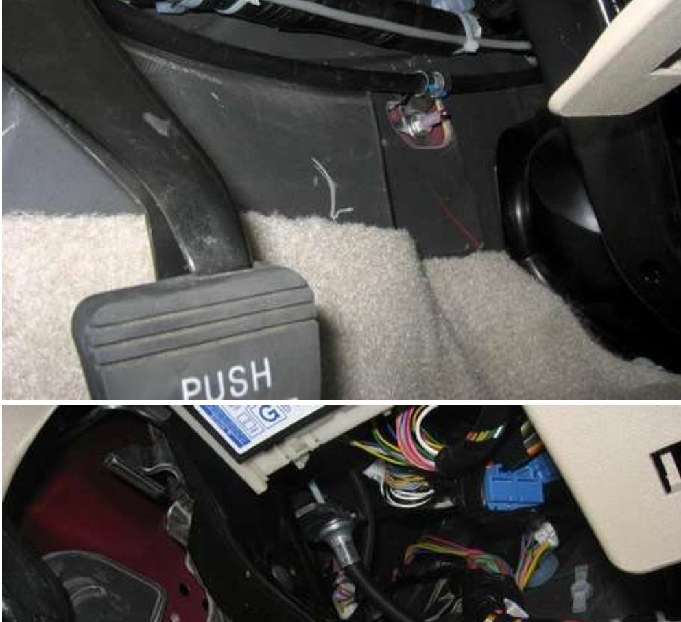
16) Cable runs behind parking brake and attached to a cable bundle
