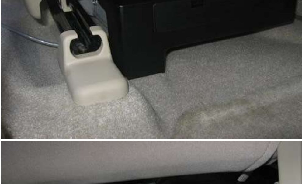
6) In this mounting position, the DB15 connector now reaches to the front of the NAV box. Note that the rear edge of the CAN-View box must be all the way to the rear of the NAV box, so that the seat doesn't hit the CAN-View box when we put the seat back.
