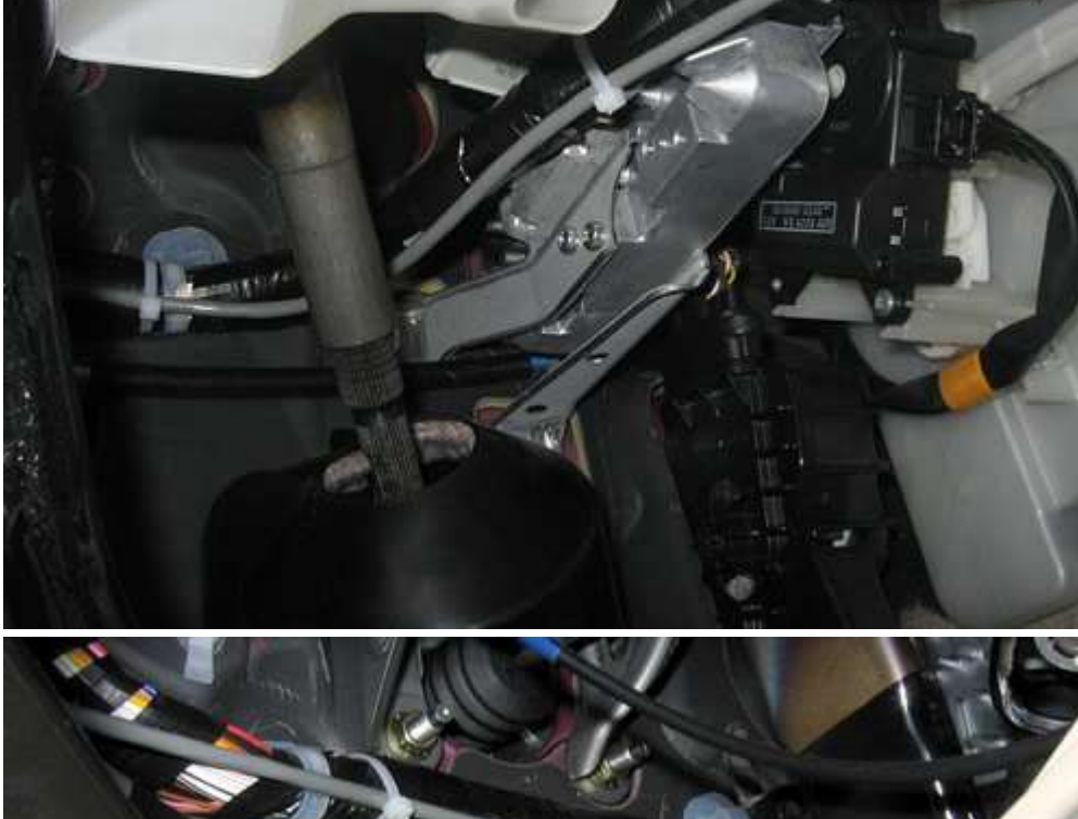
15) Routing of cable from OBD2 connector behind steering column
