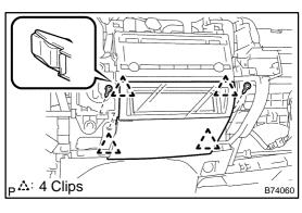
REMOVE MULTI-DISPLAY ASSY (a) Remove the 2 bolts.
