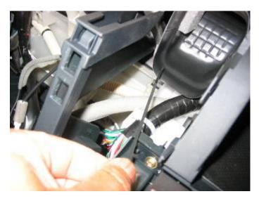
Leave enough cable to plug into the radio then tie the XM cable off with one of the zip ties located in the XM radio kit.
