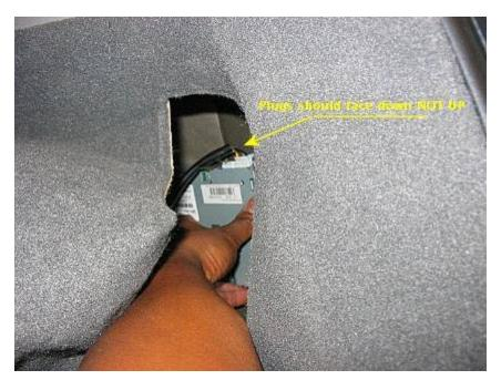
The duo-lock and XM unit will be going on the back of the exterior sheet metal (rear quarter).
