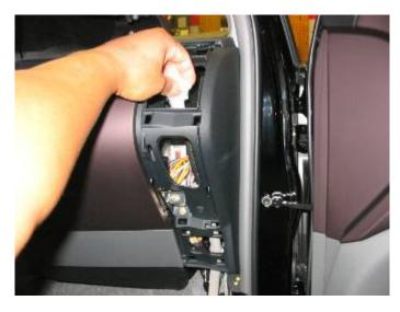
Feed the cable out of the register hole. You really only need to pull enough cable to make it to the radio assembly.
