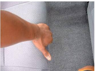
Once the clips are disengaged, pull the seat forward and remove it from the car.
