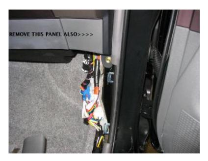
Take the cable from the XM radio kit foam side first and feed it behind the dash.
