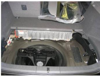
Remove right rear floor board panel. Remove upper panel.
