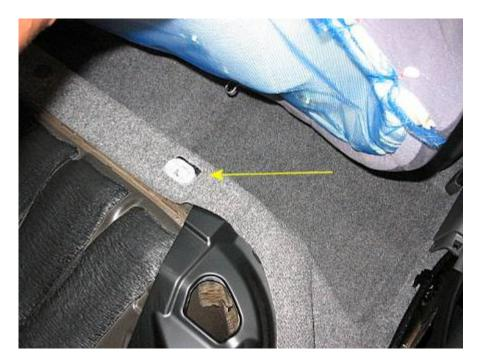
Grasps the lower front of the seat and with a quick snatching motion, pull the seat up and out of the clips.
