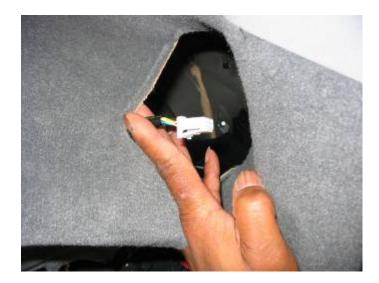
Take the XM radio unit and attach the duo lock tape from the kit to it. Plug the cable into the unit then mount the unit to the right quarter panel.
