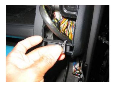
There is a special cable tie in the kit. It has sticky tape attached to it. Put the XM cable into the tie then stick the tie to the inside of the dash by register No.4.
