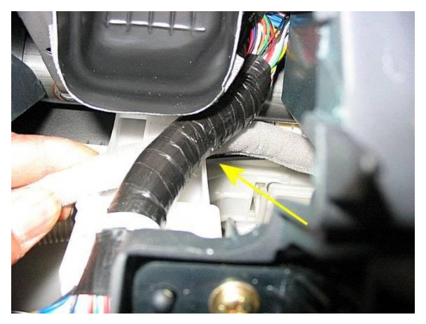
Make sure to run the XM radio cable under this bundle of wires.
