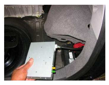
Make sure your plugs are facing down and not up when mounting. Find the flattest surface possible. There is a prime spot just above and ahead of the battery.
