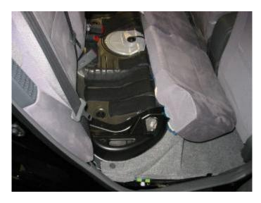
Fold down right rear seat. Remove cargo cover, spare tire cover and cargo tray. Peel back carpet (velcroed to seat back).
