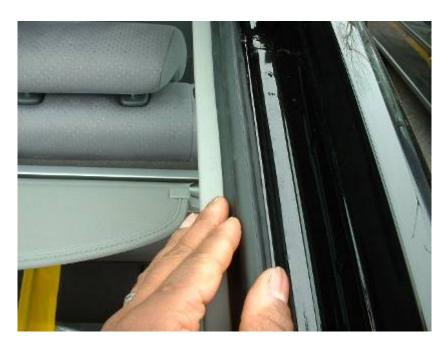
Refit all of your panels. Replace the carpeting, cargo and spare tire covers. Replace the sill plates and any other items removed.
