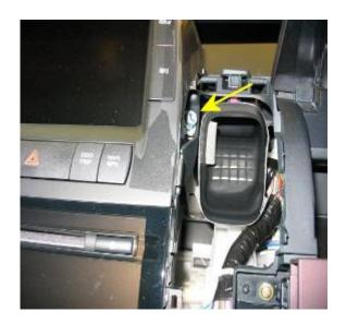
It is not necessary to disconnect the cables to the multi display. It can sit off to the side of the dash. If you feel more comfortable, you can remove the cables to facilitate removing the display from the car.
