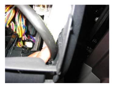
Be sure the cable is pulled taught. What we are trying to do is have the cable not interfere with the glove box door. Be sure to check it's operation and make adjustments to the cable as needed.
