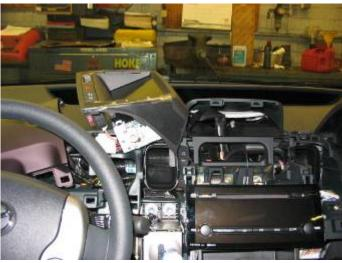
Remove radio assembly. Remove the 4 screws.
