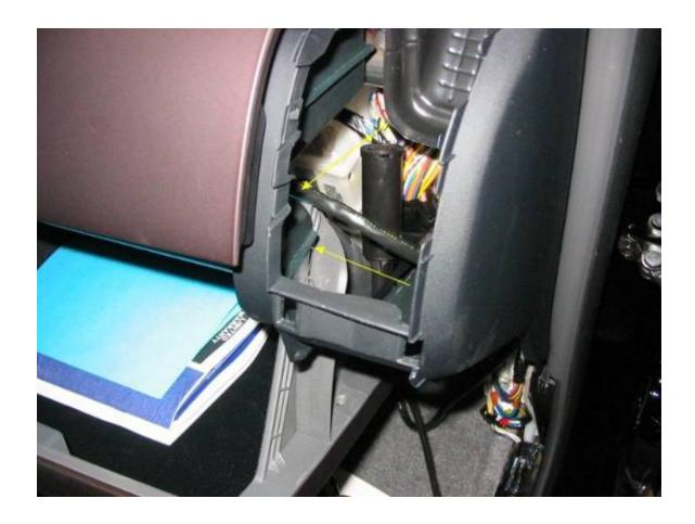
Plug the XM Radio cable into the radio. Reinstall the radio, center dash, multi display. Reinstall all dash panels and registers. Reassemble everything except the RH cowl panel and the RH front sill plate.
