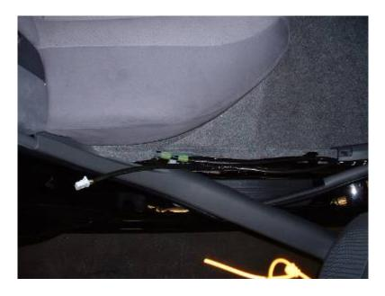
Here you will see that the rear seat is removed. It is not absolutely necessary but it is so easy to do and makes the install a little easier. The front of the rear seat pops into these plastic clips.
