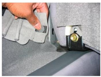
Feed the XM radio cable up behind the folded rear seat on the outside of the seat belt.
