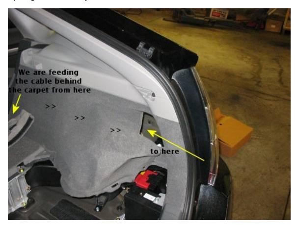
Pull the carpet liner out at the bottom, it's easier to see where the cable is being routed.
