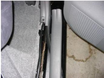
Pull the weatherstrip away from both sides of the B pillar panel (You know, that plastic panel between the front and rear doors).
