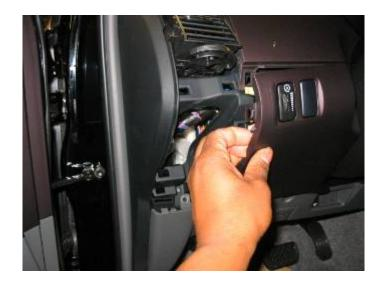
The panel is held on with the same clips as the ones for the register Grasp the panel and pop it loose.
