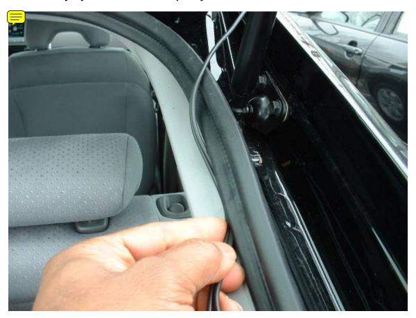
Route the antenna wire behind the right finish panel. Plug the antenna into the XM radio unit. Test the XM radio operation once again.
