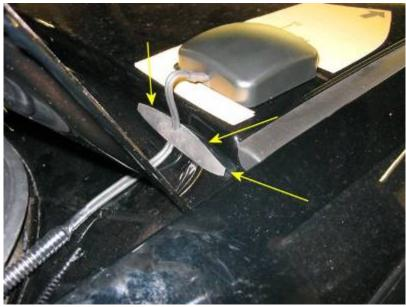
Remove the backing from the tape on the antenna wire and stick it to the car. Be sure the area is clean.
