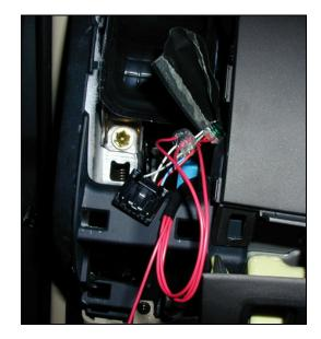
After that, I tested the EV button illumination by plugging in the dimmer to the plug, and turning on the parking lights. Success should yield an illuminated EV button which is brightness adjustable.
