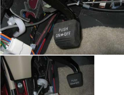
16) Cable runs behind parking brake and attached to a cable bundle
