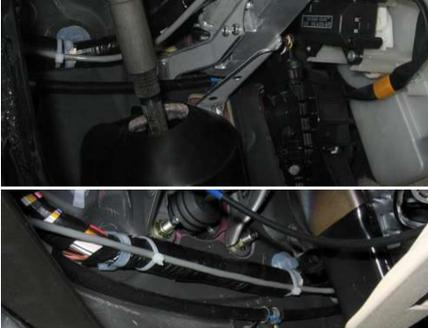
14) (right) Connected cable to the OBD2 connector and routed back
