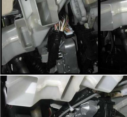
13) (left) OBD2 connector under dash to right of steering wheel
