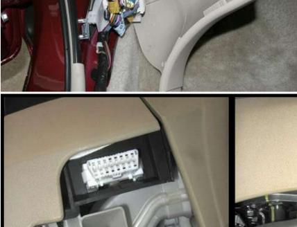
12) Driver's side kick panel removed exposes wiring
