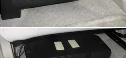
4) For completeness, here is a step that was tried and rejected: CAN-View box next to NAV box View from rear seat with front seat all the way forward. It's a tight fit getting it in but fits nice once in place. But the SCART cable won't reach and the connectors facing back would be easy to kick..
