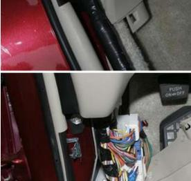
11) Remove the driver's side kick panel by pulling straight back
