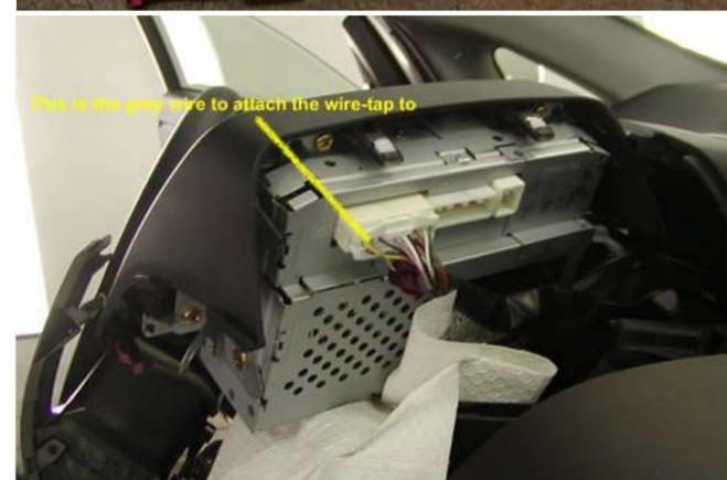
2) Next take this CAN-view cable with the plug on one end which matches the middle connector on the back of the MFD
