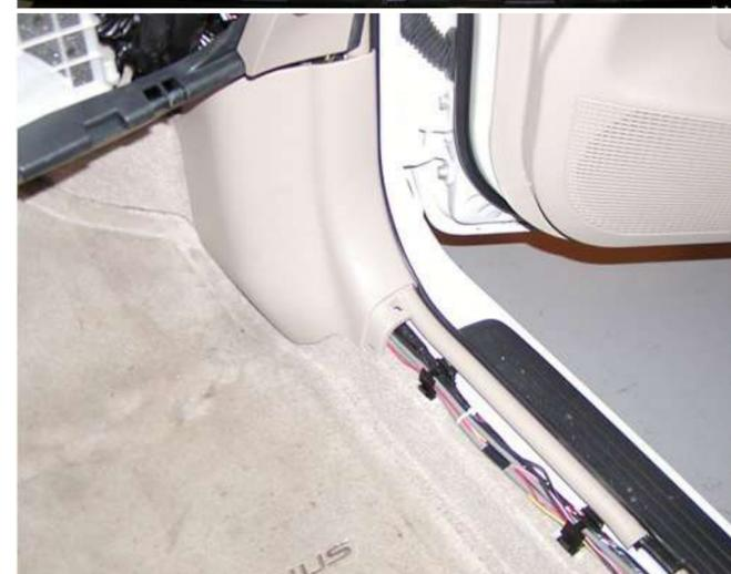
13) There is a plastic moulding from just below where the rightmost air vent was removed, down to door sill level. It is held in by more clips and just pulls out, exposing a route to follow from the back of the glove box, down to the door sill, following existing cable runs.
